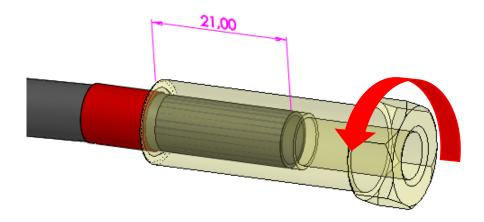
7- Screw in the male insert (clockwise) and press it against the sleeve. The hose will move back about 3 to 4 mm, which is normal.
