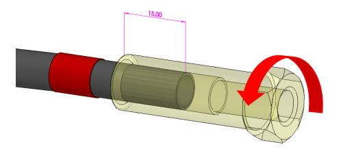
4- Lightly grease the M8 thread of the sleeve and the thread of the male insert.
