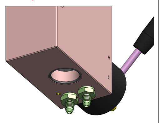
8- After changing the pump body, it is necessary to carry out a new purge (see associated procedure).
