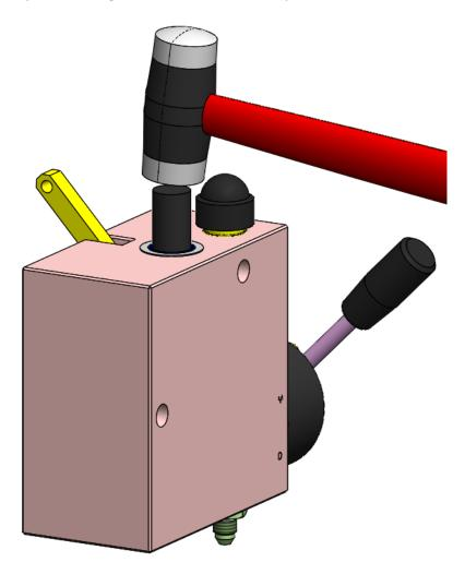
6- Completely remove the pump casing and proceed in reverse order to fit the new pump casing.
