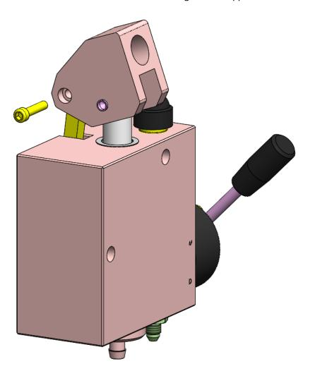
2-Remove the tipper and Ø20 piston from the top.
